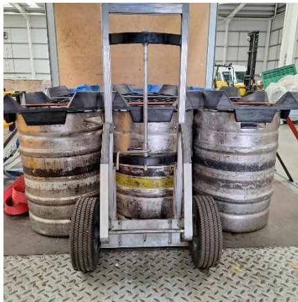
A sack trolley integrated into a secured load.
