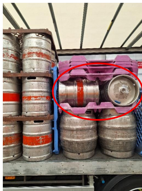
Return alternatively positioned horizontally within the locator boards. Dunnage is added either side to support a positive fit.
