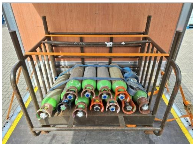
Gas cylinders are secured separately by two blue lashing straps to the gas cylinder pallet.
