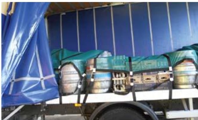
Load nets positioned over a mixed load of products, anchored to the body side rave.
