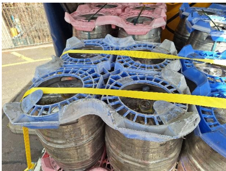
A large pack showing containers secured with locator boards and lashing straps.
