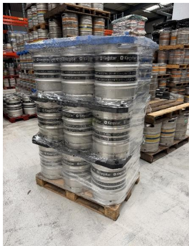
A large pack, consisting of three levels, with locator boards positioned between each level and on top, finished with shrink wrap to provide a stable load pack.
