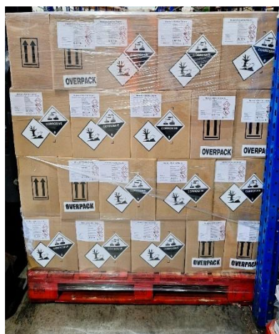
Small pack of BLC shrink wrapped to a pallet, the UN labels and 'OVERPACK' are clearly visible.
