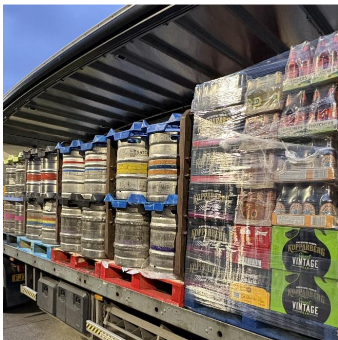
A small pack made up of boxes and drink cases, shrink wrapped to a pallet, and positioned behind large packs. A brown locator board is used as dunnage to support a positive fit within an EN12642-XL certified body.
