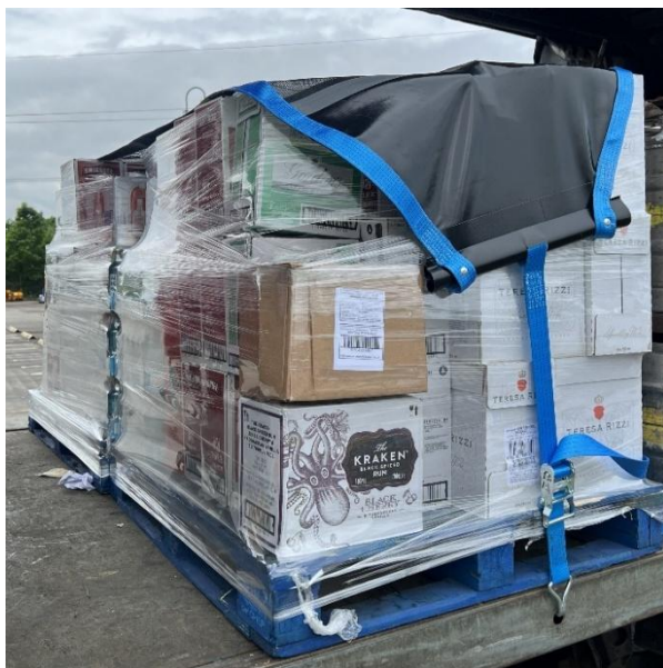
Small packs, secured with a wide lashing strap anchored to the body side rave.
