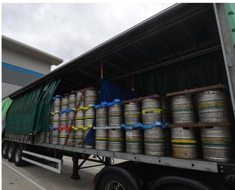
Primary distribution vehicle loaded with multiple large packs filling the load area. The body is certified to EN12642-XL and the tight packaging supports a positive fit. The higher upper level is supported by a front mounted kite mid-way down the body, together with the side nets providing auxiliary support, offering an effective load containment system.
