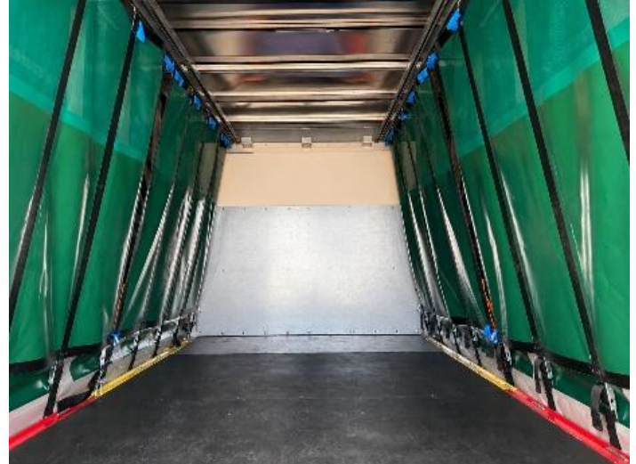
Side nets mounted from a roof rail, positioned further inwards from the curtain track. Hanging at an angle the nets provide a load hugging feature.
