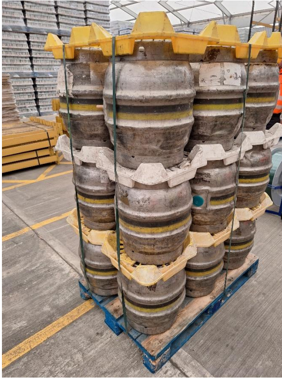
A large pack, incorporating a three level stack of containers positioned on a pallet. Locator boards are positioned in-between levels and the whole pack secured with banding to the pallet ready for loading.
