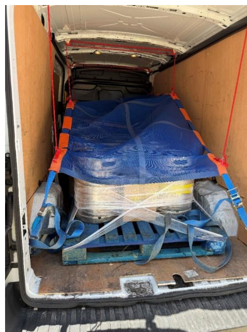
A mixed pack loaded in an LCV, secured by a roof mounted (bungee) restraint system.
