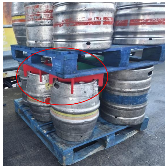
Container inserts fitted to the top of smaller containers, designed to level the support from the lower level. Note that shrink wrap needs to be applied to create a stable pack before transport as per the next image.
