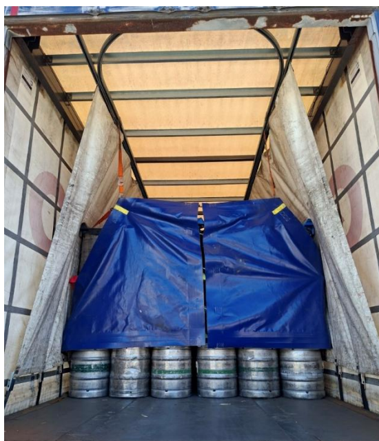
Vehicle loaded with containers, the rear mounted kite containing the load and complemented by load hugging side nets as part of a load containment
