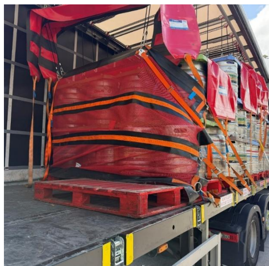
Load of large packs, secured with a load restraint system consisting of wide lashing straps over the top of the load and a rear kite securing the rear.
