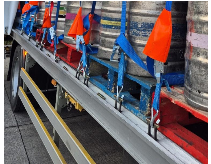
Individual lashing straps attached to individual dedicated anchorage points fitted to the vehicle body.
