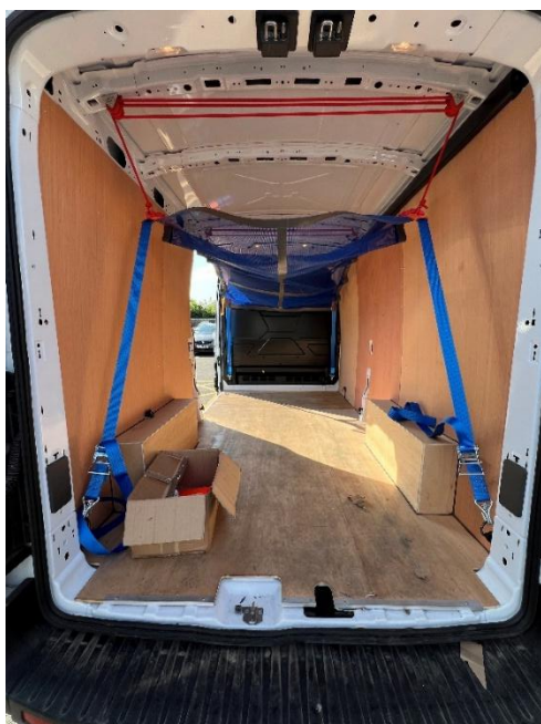
An LCV fitted with a roof mounted (bungee) restraint system ready to load.
