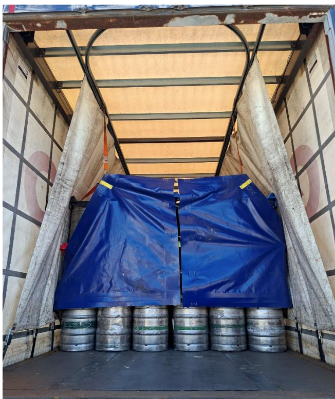
Primary distribution vehicle showing multiple large packs filling the load area with the EN12642-XL certified body providing containment. The rear kite is required to provide effective containment of the load rear, and side nets are also fitted to provide auxiliary load containment support.
