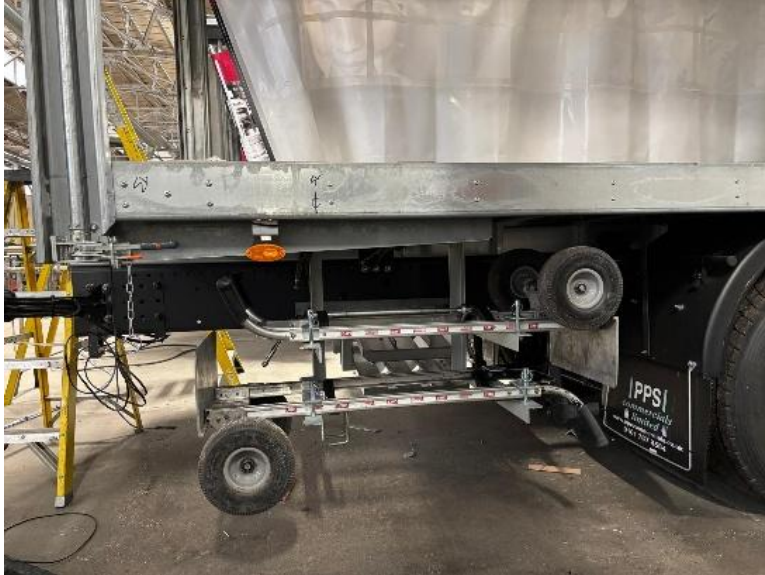
A sack trolley secured on dedicated rack system.
