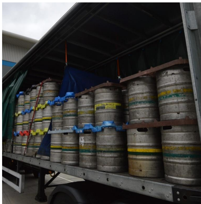
Multiple large packs uniformly distributed across the load area.
