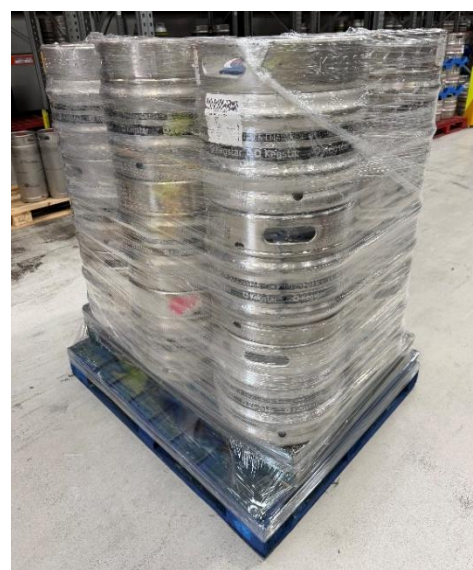
A large pack consisting of three levels using kegs specifically designed to be stacked together. Finished with shrink wrap this method forms a stable load pack. An exception to the 'no chimney stacking' rule, this method is only suitable for kegs of the exact same type and size that are specifically designed to be stacked this way.
