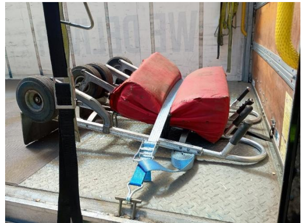
Two sack trollies and a drop mat secured to load floor with lashing strap.
