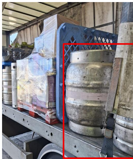
Single containers of differing sizes positioned together with the rear kite secured to support a positive fit.
