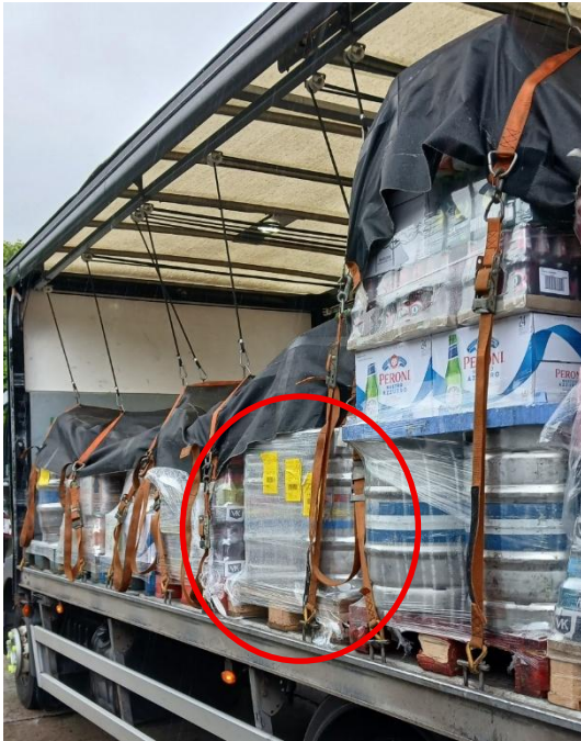
A large pack consisting of three different customer products loaded on one pallet. Note packs of similar heights are positioned together at the front to reduce the height differences and improve the effectiveness of the roof mounted (bungee) load system.
