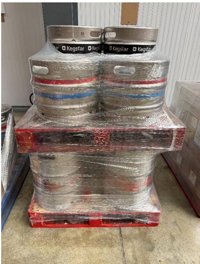
A completed stable large pack consisting of different height containers. Container inserts are fitted (not shown), the next level of pallet and containers added, and the whole load pack shrink wrapped ready for transport.
