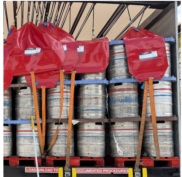
Large packs with roof mounted (bungee) wide lashing straps positioned and ready to be tensioned.
