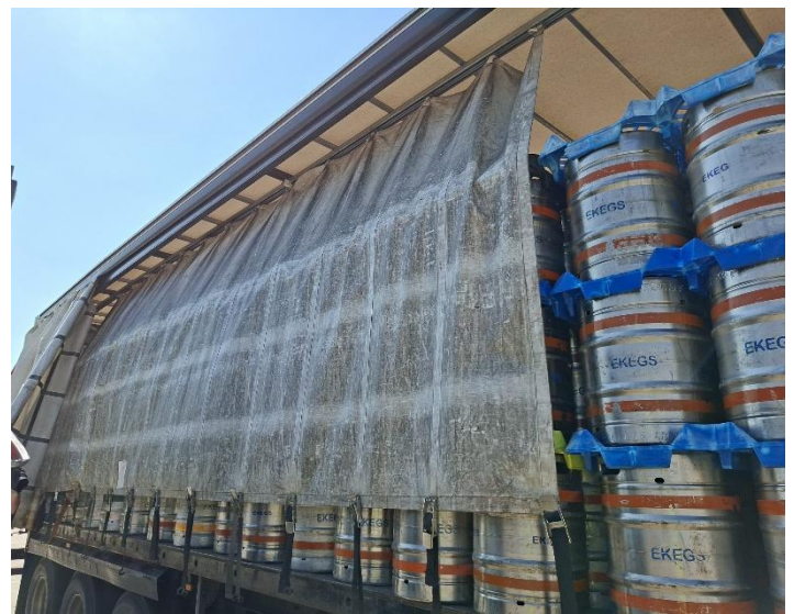
A similar design, this EN12642-XL certified body has side nets which reduces the potential risk of loads falling from the vehicle when the curtains are opened. Note that if the vehicle body was not constructed to EN12642-XL a load restraint system would need to be employed to provide satisfactory load security.
