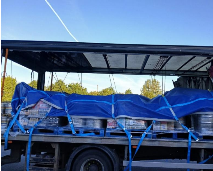
A mixed load secured with a load net (roof mounted (bungee) load system shown, see below).
