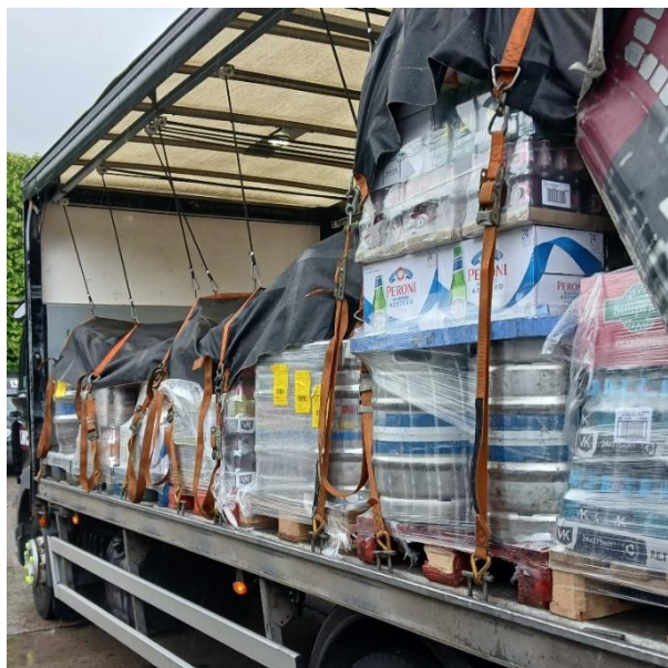
Load planned in drop order, single packs utilised at the front to manage weight distribution as load diminishes from the rear.
