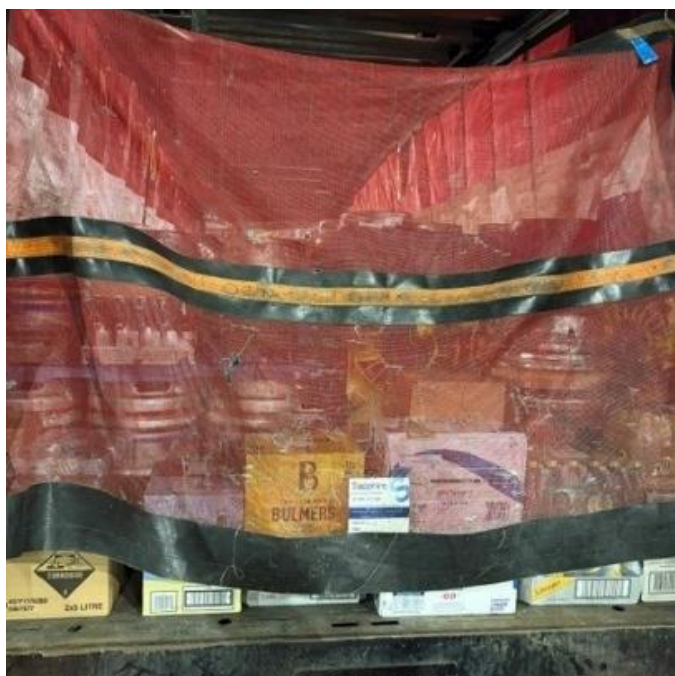
A rear kite un-tensioned during a short journey within an urban environment, not exceeding 30mph. All products are positioned in a safe location on the vehicle and will stay put. Note the outer doors and curtains would be secured closed to provide containment.
