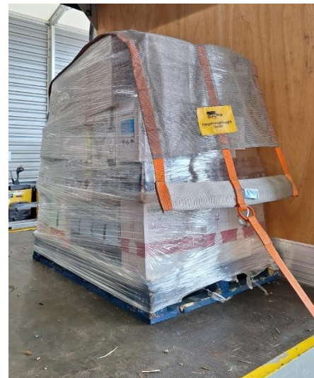
A single small pack secured with a wide lashing strap.
