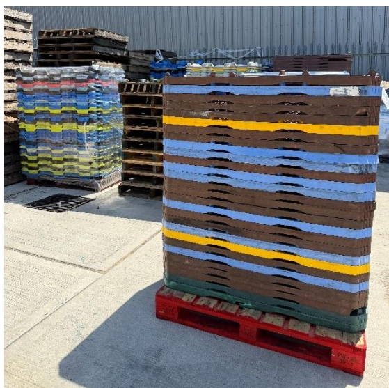
Stacks of different locator boards, designed to fit different sizes of container. They should not be held longer than is necessary.
