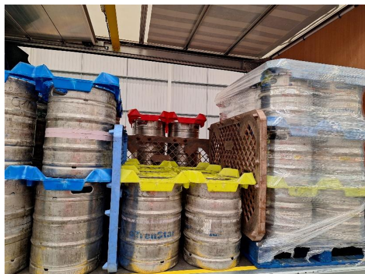
Secondary distribution vehicle loaded with different levels of packs; one large pack is shrink wrapped and all supported by the use of locator boards. The tight packaging of the load eliminating gaps, and use of an EN12642-XL body, supports a positive fit and provides an effective load security solution.
