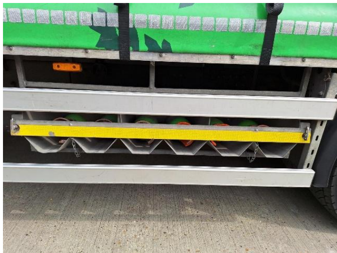
Gas cylinders mounted in a specialised rack with the valves positioned uppermost. The detachable retaining rail is secured to ensure the cylinders stay put during transport.
