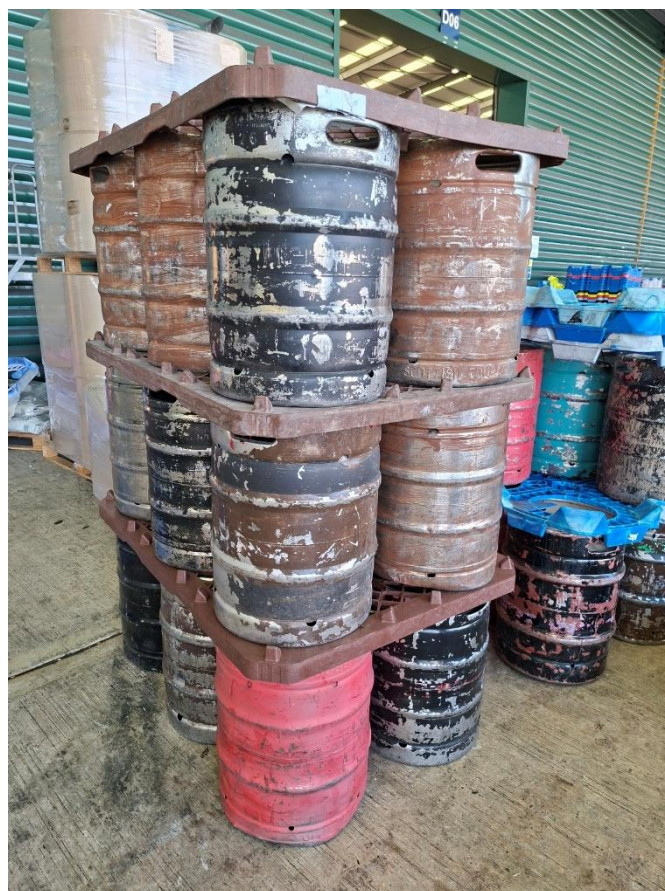
Dummy containers painted differing colours for identity, used when constructing loads to round up container odd numbers to support a positive fit.
