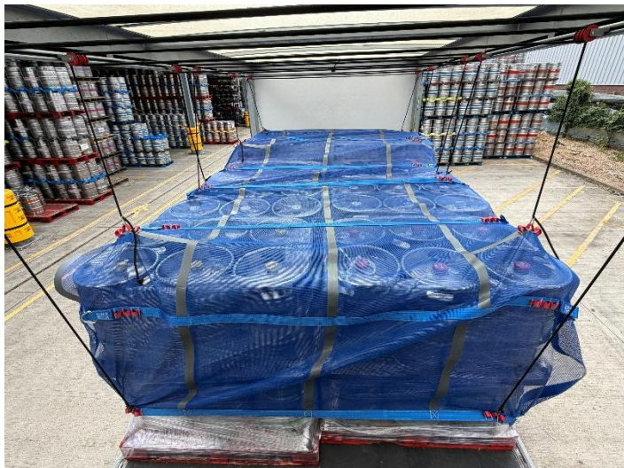
A load consisting of small packs at the front and large packs at the rear, uniformly distributed across the load area. Load security is achieved using a roof mounted (bungee) restraint system.
