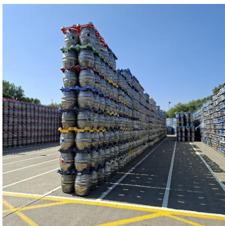
Empty containers on site, stacked with locator boards, demonstrating good static stability.
