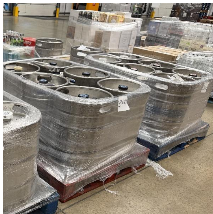
Containers shrink wrapped to a pallet to provide a secure large pack.
