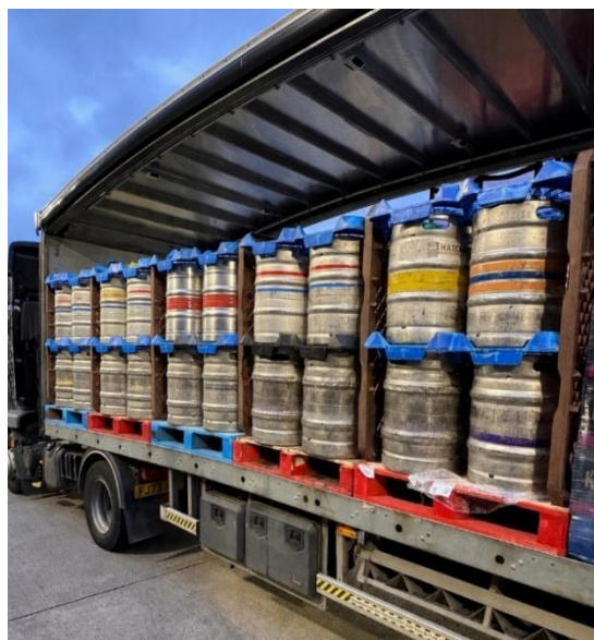
A load consisting of large packs, uniformly distributed across the load bed, with locator boards used as dunnage to support a positive fit within an EN12642-XL certified body.
