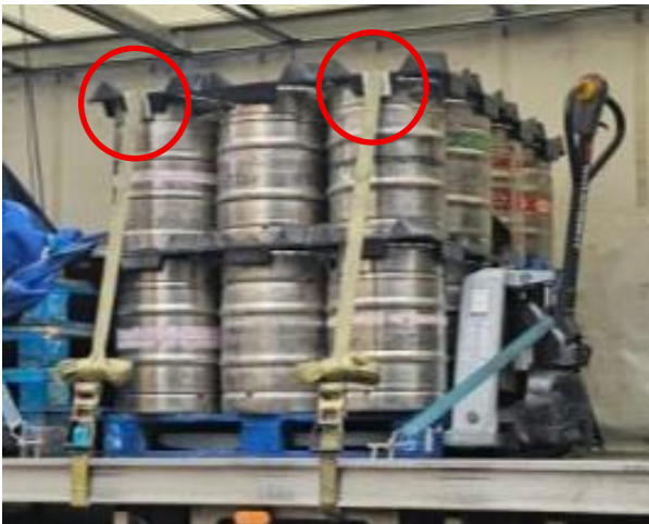
Large packs secured with lashing straps, fitted with edge protection to protect the webbing and locator boards.
