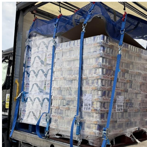
Two small packs, each pack consists of one product type. The load is shrink wrapped to the pallet with a roof mounted (bungee) restraint system positioned ready to be pulled down and secure the load.
