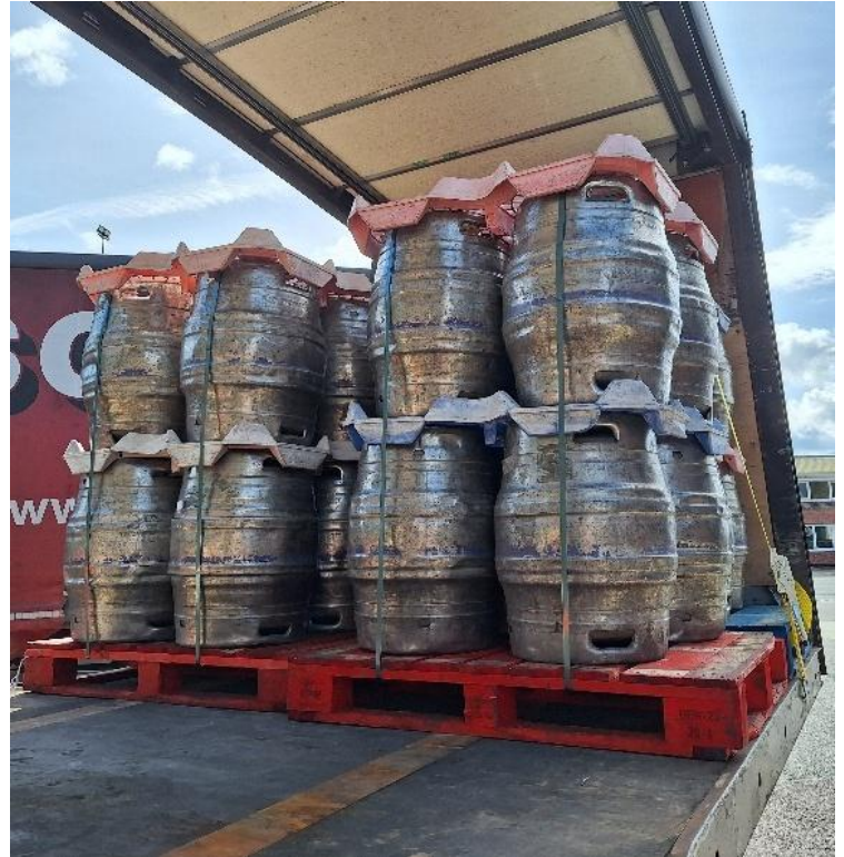
Two large packs incorporating two level stacks of containers positioned on pallets. Locator boards are positioned in-between levels, and each pack is secured with banding to the pallet. The packs are then secured to the vehicle load bed by lashing straps.
