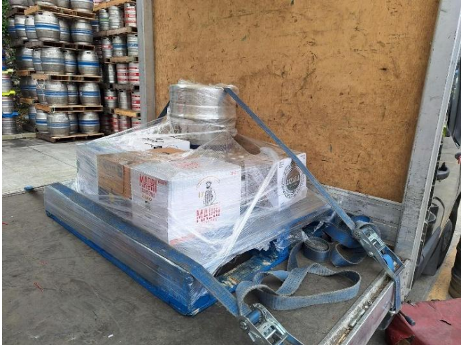
A mixed pack consisting of an individual container and other retail products, shrink wrapped to a pallet and secured to the vehicle using lashing straps. Note that only shrink wrap is securing the boxed retail products to the pallet, the shrink wrap needs to be of adequate strength/thickness to fulfil this function.
