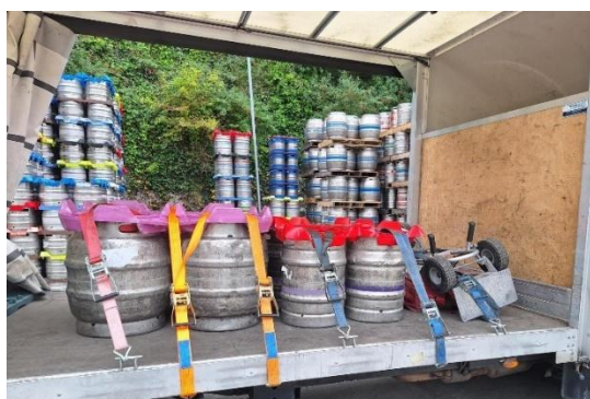
A curtainsided LCV loaded with a single layer of containers and sack trolley. Locator boards are fitted and the whole load secured with lashing straps.
