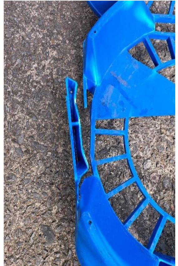
A damaged locator board, affecting the structural integrity and requiring replacement.
