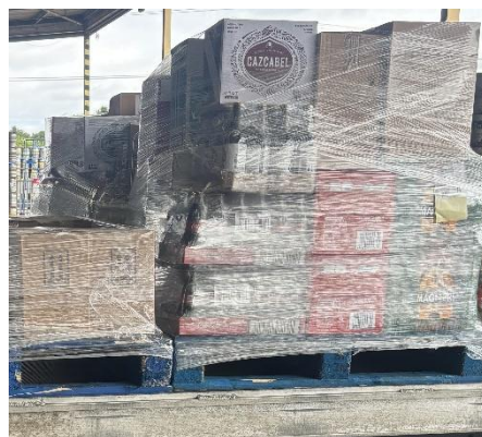
A small pack consisting of individual product packages stacked on a pallet, the whole pack is secured with shrink wrap to provide a stable pack prior to load restraint systems being applied.
