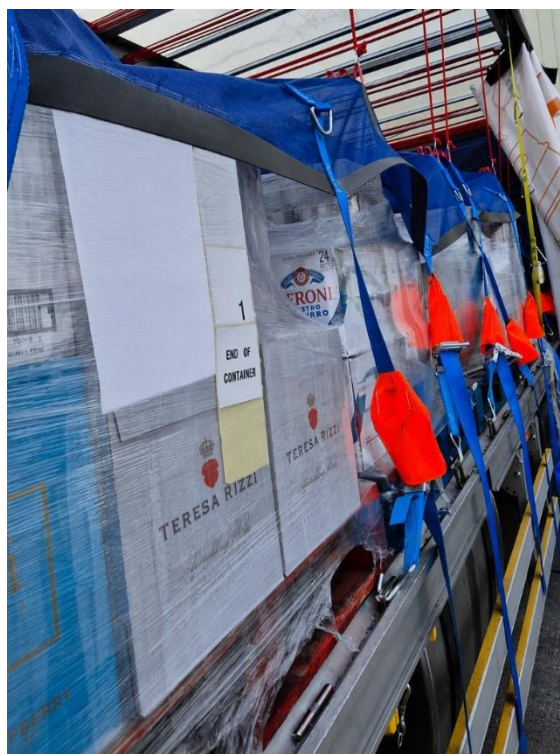
Multiple consignments uniformly distributed for multidrop operations.
