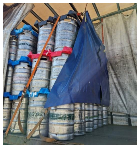
Large packs stacked using locator boards, secured at the rear by a kite anchored to the side rave to support a positive fit and effective load containment system.
