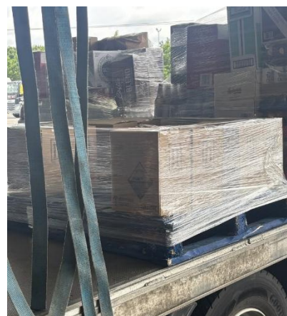
Small pack of BLC loaded on vehicle, a roof mounted (bungee) load system will be positioned and secured prior to transport.
