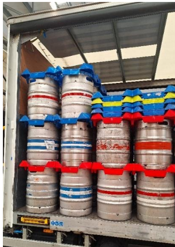
A three level stack of empty containers, using locator boards in-between and on top, is loaded against the headboard. The two level stack behind is topped with five locator boards to increase the effective height of the lower load, helping to retain the upper items and achieve a positive fit. Note more locator boards may be required to support larger/heavier containers.
