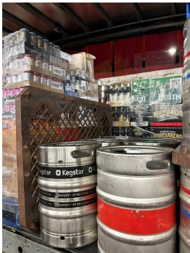
Single containers, contained within the load area by other products and dunnage supporting a positive fit.
