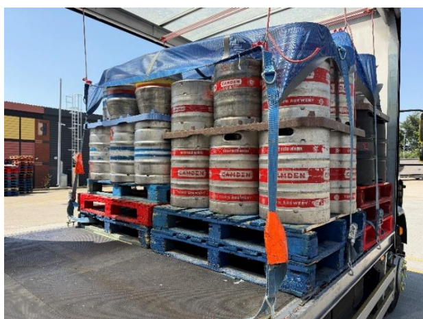
Empty containers being returned through reverse logistics. Secured by a bungee mounted load net system; lowered, secured and tensioned to provide good load security.
