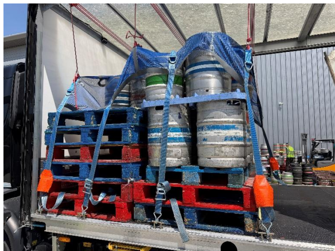
Containers and pallets being returned to the hub. Load security is achieved utilising a roof mounted (bungee) restraint system and lashing straps to provide an effective load restraint system.
