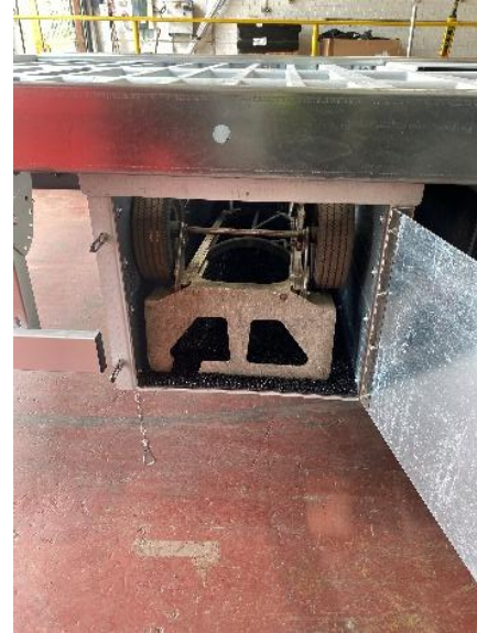
A sack trolley stowed in a bespoke chassis mounted container.
