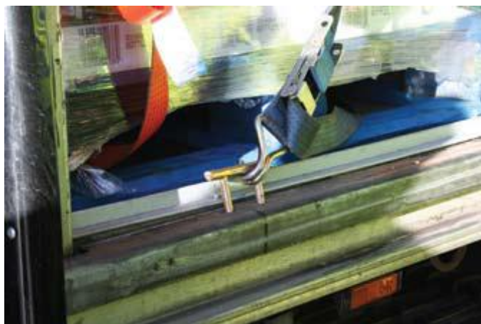
A lashing strap attached to a dedicated anchorage point fitted to the vehicle.
