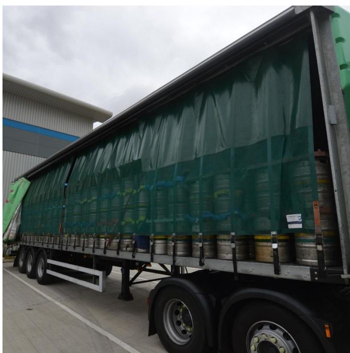
The body is constructed to EN12642-XL providing the principal load containment system. The load is uniformly distributed and fills the width of the load area supporting a positive fit. Also fitted are side nets providing auxiliary load containment support.
