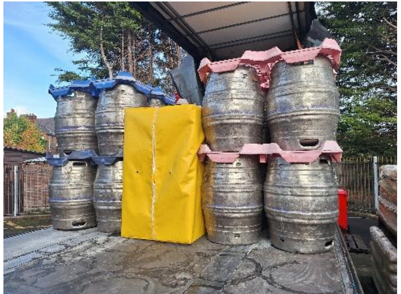
A compressible void guard inserted between two large packs to remove the gap and support a positive fit.
