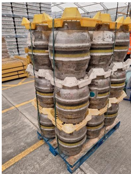
A large pack consisting of containers stacked on a pallet. Locator boards are positioned between the levels and on top, the whole pack is then secured with banding to provide a stable pack.
