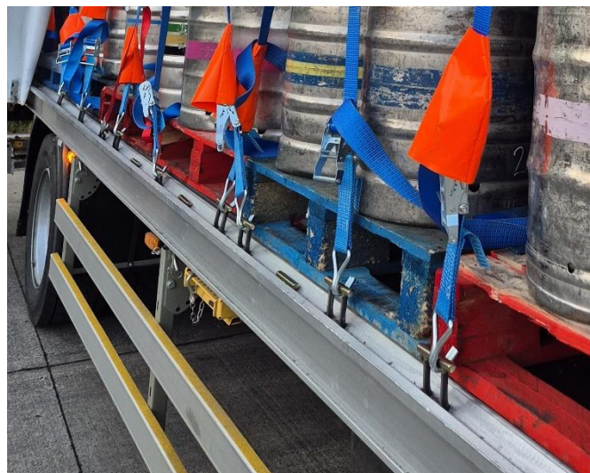
Individual lashing straps attached to individual dedicated anchorage points fitted to the vehicle body.
