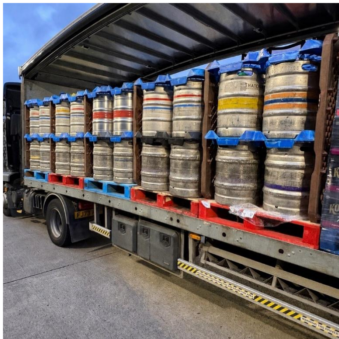
Secondary distribution vehicle loaded with large packs on pallets, utilising locator boards to provide stability. The EN12642-XL certified body and tightly packaged load (positive fit) support an effective load containment system.
