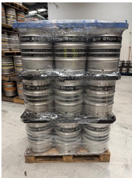
Containers stacked on a pallet. Locator boards are positioned between and on top, the whole pack is secured with shrink wrap to provide a stable pack.
