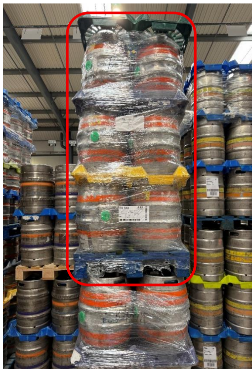
A three-level large pack of containers, utilising locator boards for stability, used in conjunction with a pallet and shrink wrap to form a stable load pack.
