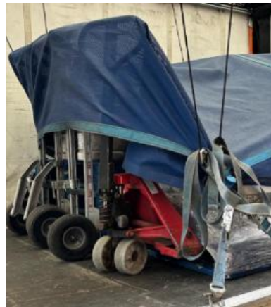
A sack trolley and pump truck integrated into a secured load.
