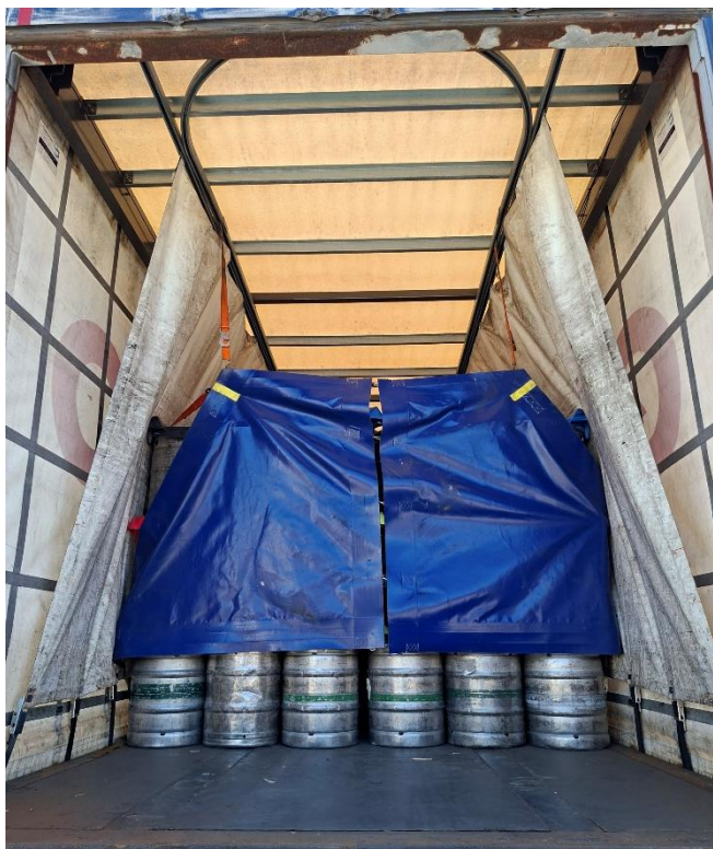
Primary distribution vehicle showing multiple large packs filling the load area with the EN12642-XL certified body providing containment. The rear kite is required to provide effective containment of the load rear, and side nets are also fitted to provide auxiliary load containment support.
