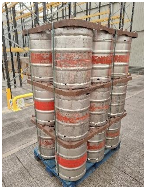
A large pack of containers, stacked to three levels on a pallet, locator boards positioned in-between and secured with banding.
