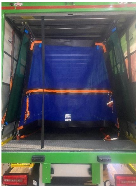
Empty vehicle showing rear mounted kite, complemented by load hugging side nets as part of a load containment system.
