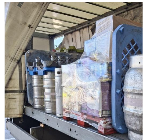
Small packs and individual containers assembled along with locator boards to provide a positive fit.
