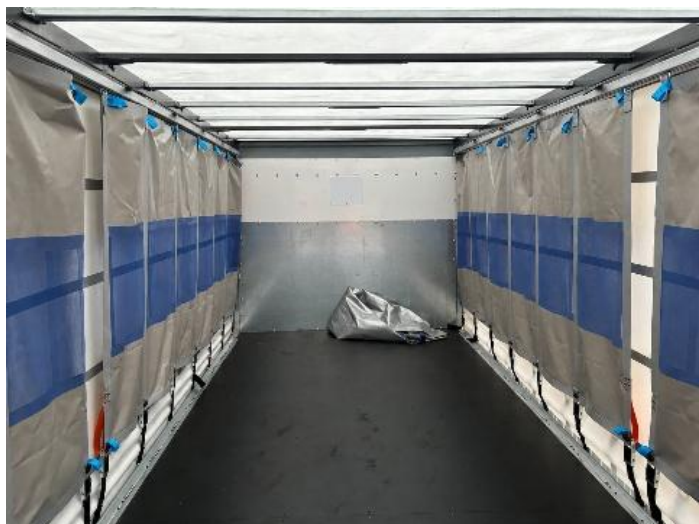
Side nets mounted from a roof rail, positioned inwards of the curtain track, hanging vertically with the bottom secured at the load floor level.
