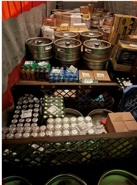
The load area is compartmentalised; load security is achieved using load containment systems.
