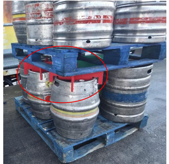
Container inserts fitted to the top of smaller containers, designed to level the support from the lower level. Note that shrink wrap needs to be applied to create a stable pack before transport as per the next image.
