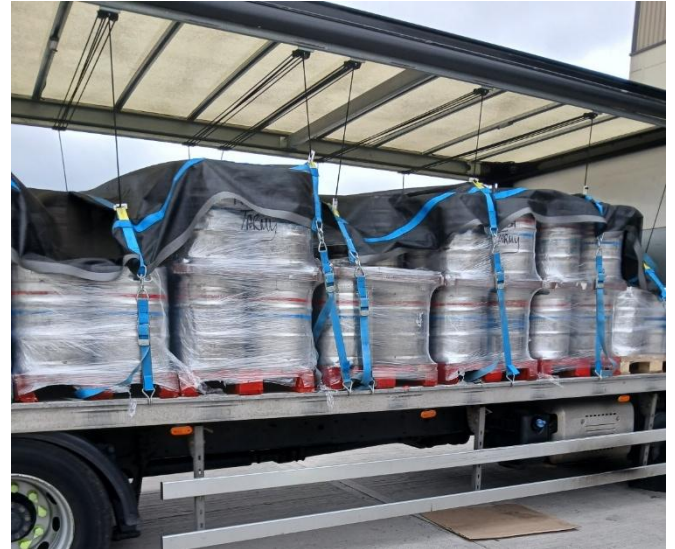
A load of large packs secured with a load net (roof mounted (bungee) load system shown, see below).
