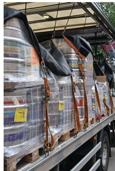
Single and two level stacks of containers on pallets, separated by locator boards and the top secured with a roof mounted (bungee) restraint system.
