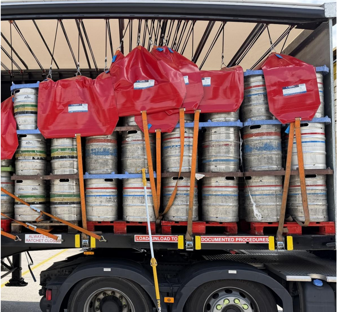
A load of large packs with wide lashing straps, suspended by bungee load system, positioned ready for tensioning.
