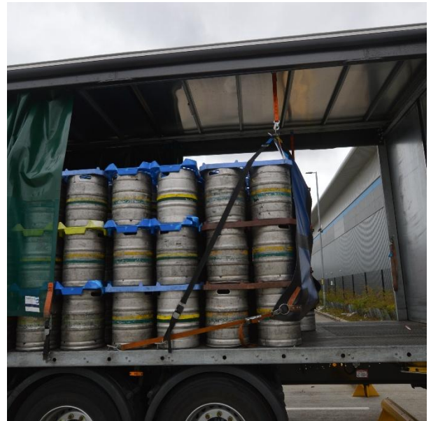
Large packs stacked using locator boards, secured at the rear by a kite anchored to the side rave supporting the load containment system.
