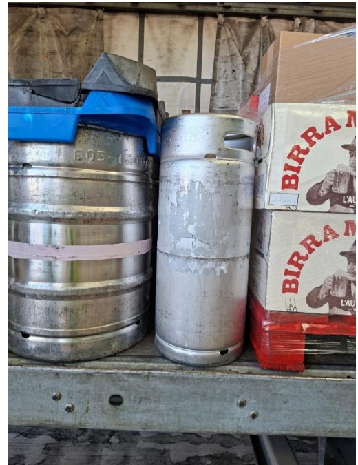
Small containers positioned into the load, filling the gap between larger containers and a small pack, supporting a positive fit.
