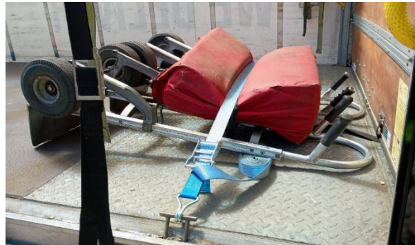
A drop pad (and sack trolley) secured to the load carrying area.
