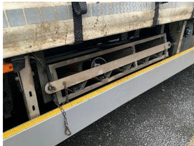
A specialised gas cylinder rack fitted to the vehicle with the retaining device in place (un-latched), ready for removal for cylinder access.
