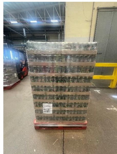
A small pack consisting of product packages stacked on a pallet, lock and pop is applied between the packages and the whole pack is secured with shrink wrap to provide a stable pack.
