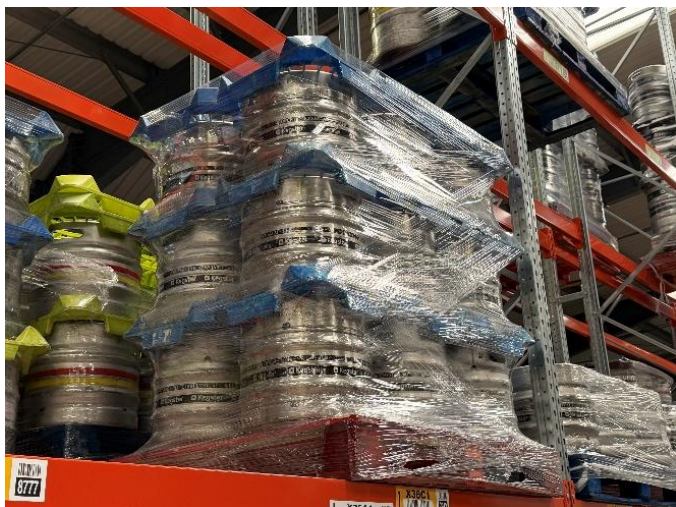
Large packs positioned in warehouse racking, consisting of varying numbers of containers, shrink wrapped to pallets with locator boards positioned between levels.
