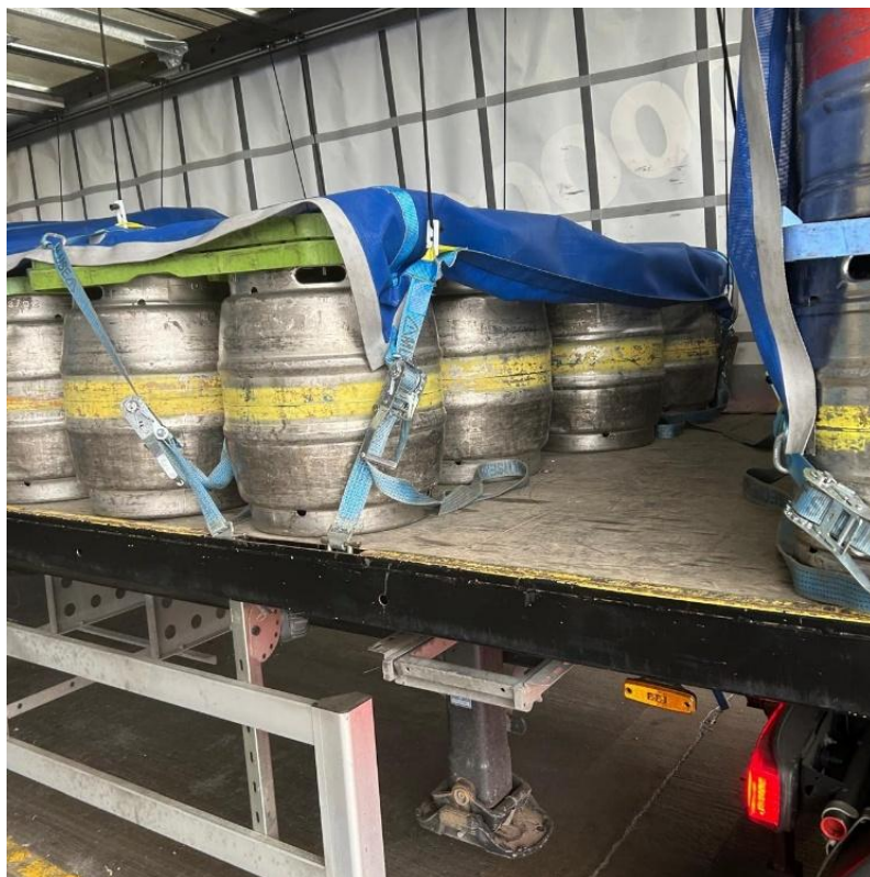
Single containers showing locator boards positioned on top and restrained using a roof mounted (bungee) restraint system.
