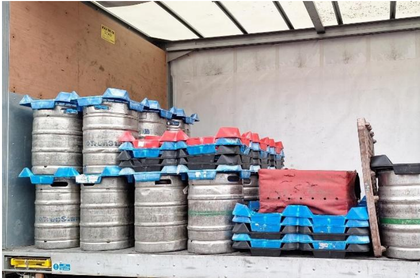
Locator boards positioned to remove gaps supporting a positive fit. Note a minimum of five must be used horizontally to provide sufficient structural strength to be effective, more may be required to support larger/heavier containers.
