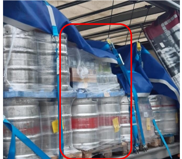
A mixed pack in between two large packs. The lower level consists of containers, the upper level consists of assorted drink cases, all shrink wrapped to a pallet and secured using a roof mounted (bungee) restraint system.
