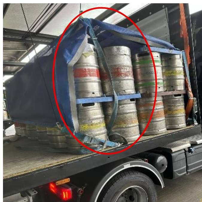
An un-tensioned lashing strap and top locator board removed to allow access to the containers. Note the curtains would be closed and secured to provide containment for a short journey in a small geographical area at low speed.
