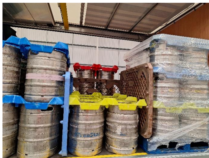
A full undelivered large pack is positioned up against the headboard, with empty containers stacked behind. Load security is achieved utilising locator boards and dunnage to support an effective positive fit.
