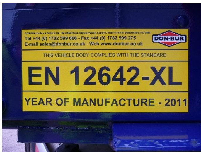
Pre 2016 example label indicating the body construction standard.
