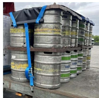
Large packs secured with locator boards and a wide lashing strap, anchored to the body side rave.
