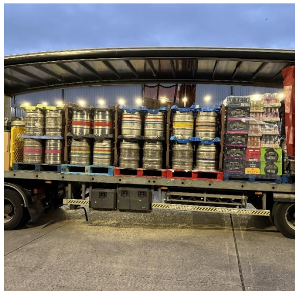
Load planned in drop order from the rear. Full containers will be swapped out for returns to maintain a positive fit throughout the journey.
