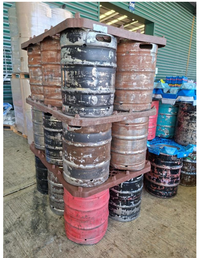
Dummy containers painted differing colours for identity, used when constructing loads to round up container odd numbers to support a positive fit.
