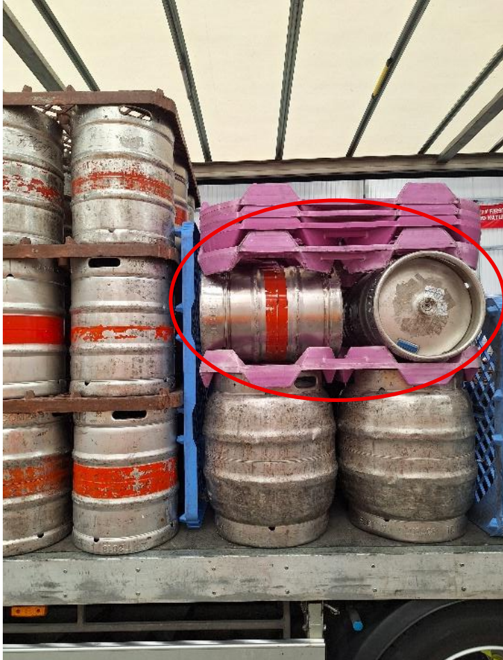
Different sized return containers stacked horizontally within two locator boards, see reverse logistics for more information.
