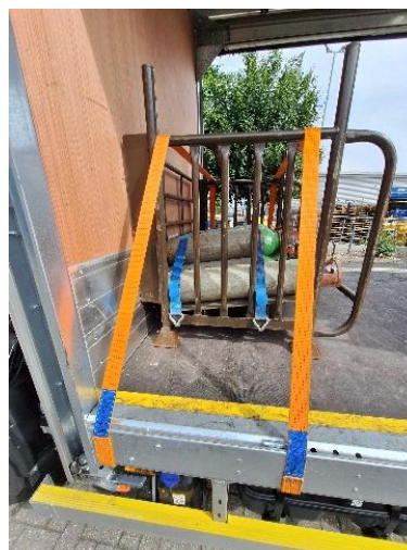
The gas cylinder pallet is secured separately to the load floor with two yellow lashing straps.
