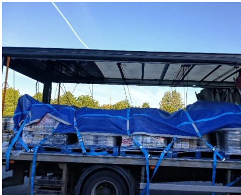
Individual small packs and mixed packs are loaded together. Load security is achieved over the differing consignment heights using a roof mounted (bungee) restraint system.
