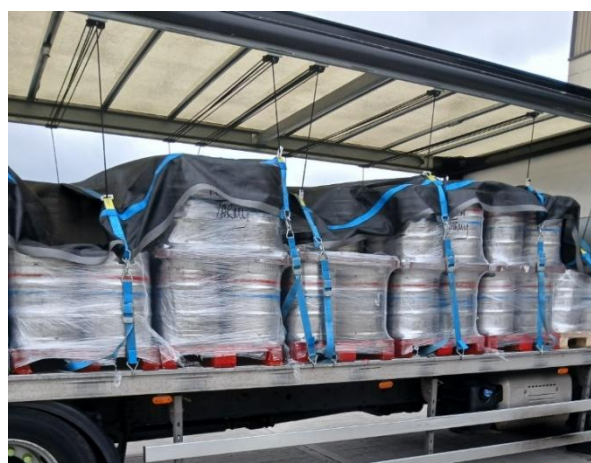
A load of large packs secured by a bungee mounted load net system. Lowered, secured and tensioned to provide good load security.
