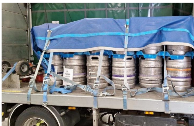
Two levels of containers, locator boards are positioned between levels, the load is secured with roof mounted (bungee) restraint system and lashing straps anchored to the side rave (dedicated anchorage points not fitted).
