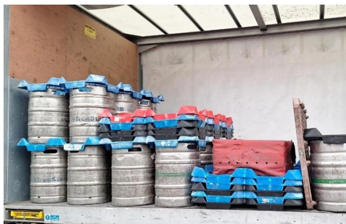
Returns are loaded from the headboard. Locator boards are used not only on top of containers to help manage horizontal movement, but also vertically and stacked horizontally as dunnage. Note a minimum of five locator boards are needed to provide sufficient support when used horizontally as dunnage, more maybe required to support larger/heavier containers.
