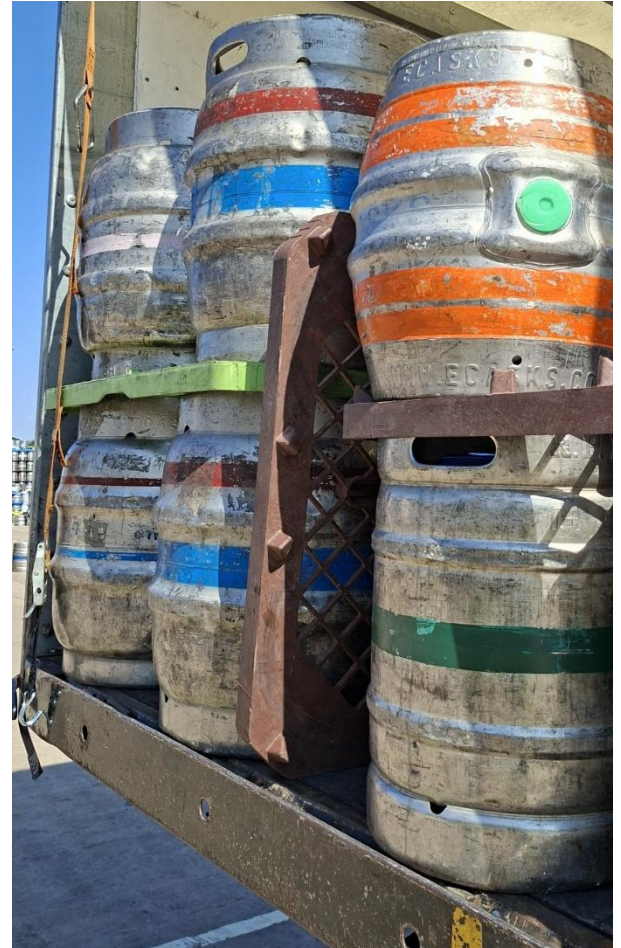
Different sized return containers stacked, positioned close together and using locator boards as dunnage to support a positive fit.
