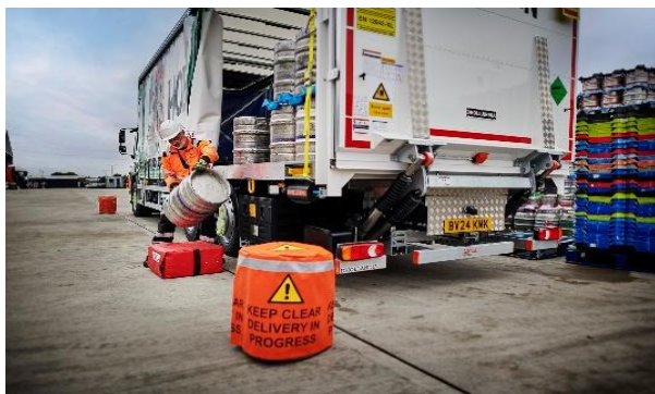
A drop pad in use during the manual unloading process.
