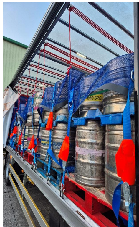
A load of large packs secured by a bungee mounted load net system; lowered, secured and tensioned to provide good load security.
