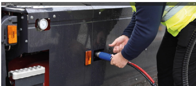
Fig 4: Refuelling of CNG vehicle
