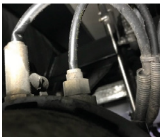
Fig 4: Kinked brake pipe
