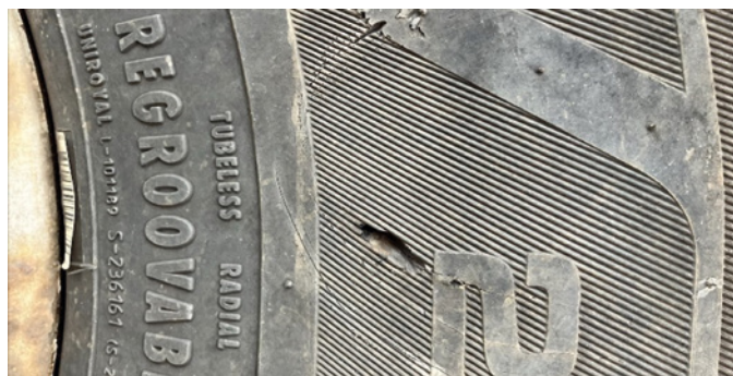
Fig 8: Tyre wall damage
