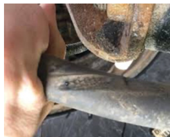
Fig 5: Damaged brake hose
