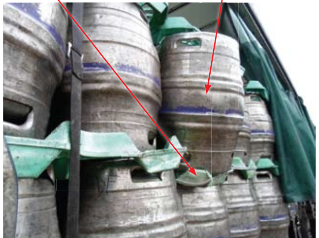
Locator board in poor condition which is likely to have caused the shifting of the load, causing the upper barrels to become unstable
