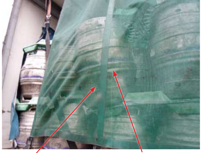
Locator board in poor condition which is likely to have caused the shifting of the load, causing the upper barrels to become unstable
