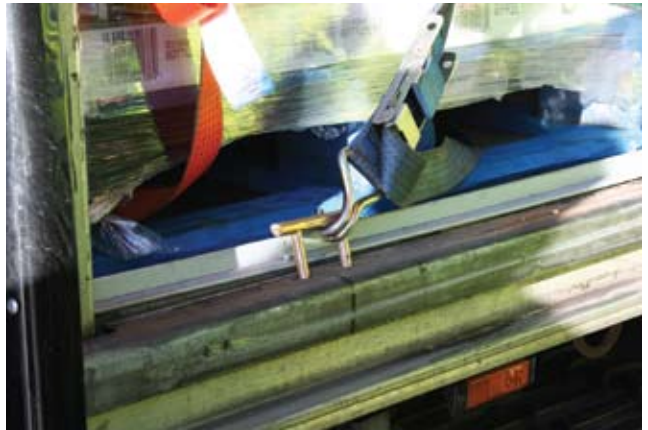
Dedicated load restraint points should be used (where fitted) as these provide the best method of attachment for straps
