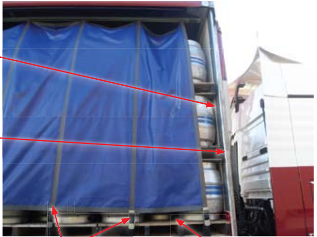
Inner containment curtain rail is in good order and condition, strapping attachment is in good order
