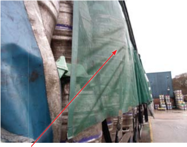
Evidence of load shift. Possible prohibition action by VOSA would result
