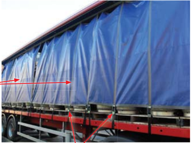
Condition and number of straps and buckles is adequate
