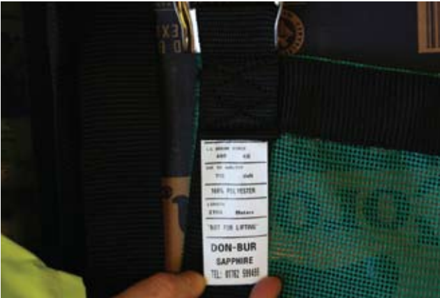
Example of retaining strap load rating label
